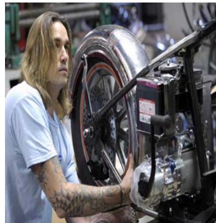
Voodoo Choppers owner Eric Gorges of Clarkston test fits the rear fender on a custom-built chopper with a kick starter. (Todd McInturf / The Detroit News)
